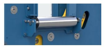
**Guide rollers** We supply high-quality rollers for the KNOF, for guiding the bars into the machine.
